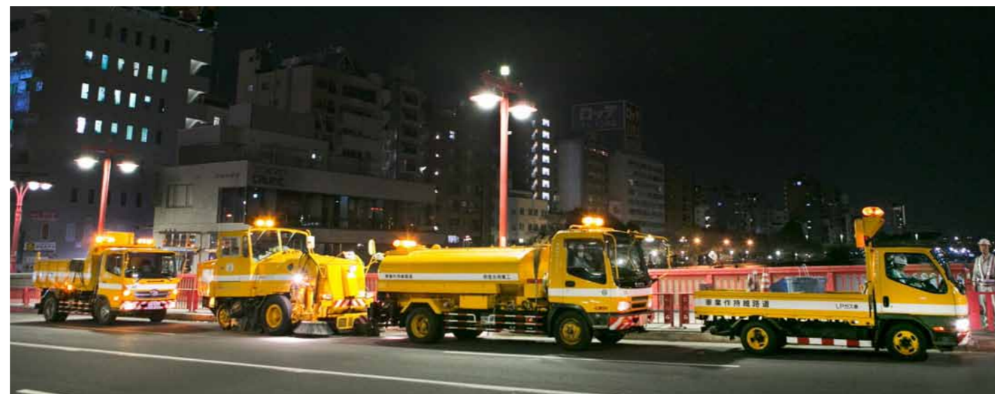
The road-cleaning team lines up for work. From right, the lead vehicle, sprinkler truck, sweeper, and dump truck.
