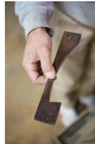
For round-shaped tubs, you use precision guides when chiselling the wood.
