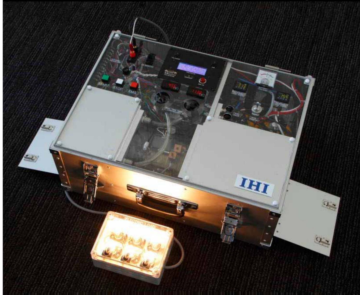
In addition to the turbine placed in the front center, the photo also shows the fuel feed (upper right), the controller (upper left), and an air inlet and a noise canceller to the right of the turbine and another noise canceller on the left. The entire system including the case weighs about 13 kilograms but further miniaturization will reduce the size of the case by half and slash the weight to eight kilograms.
