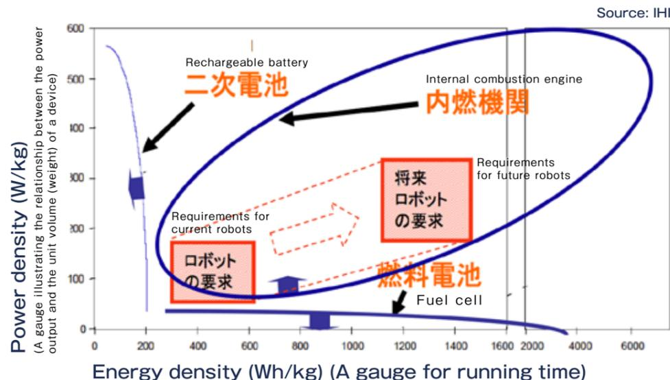
Neither rechargeable batteries nor fuel cells can fully satisfy the dual requirement of high current and long running time needed for robots. All internal combustion engines, including gas turbines, can satisfy the dual requirement. However, gas turbines emit no exhaust gas, making them the most promising solution for use in sealed environments such as indoor areas.
