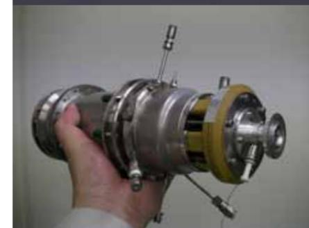
The main body of a palmtop gas turbine. A power output of 400W and rotation speed of 400,000 RPM is achievable. In addition to propane gas, it has run successfully on light oil and kerosene. Theoretically, bio fuels could be used as well. The photo on the left shows a gas turbine with a heat exchanger, which elevates the heat efficiency to a level equivalent to that of a gasoline-powered engine.
