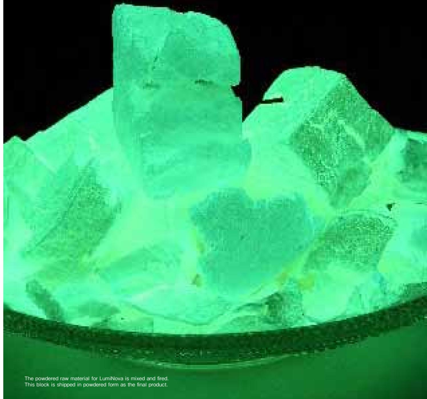
The powdered raw material for LumiNova is mixed and fired. This block is shipped in powdered form as the final product.
