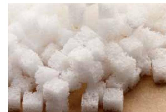
One centimeter blocks of PVA. Its water absorption and retention capabilities are excellent, as is its abrasion resistance. The idea of purifying water by housing microorganisms in holes is currently undergoing verification.
