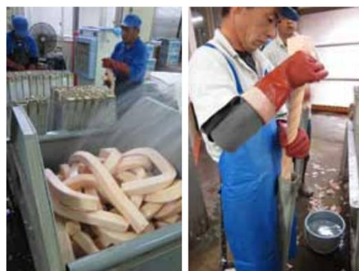
The Tsukuba plant and two overseas factories in China and Thailand together produce over fifteen million sponges every month. The material is poured still foaming into a mold, steamed, then removed from the mold by twisting up with two hands. This work must be performed by hand since the material is too soft to be handled by machines.
