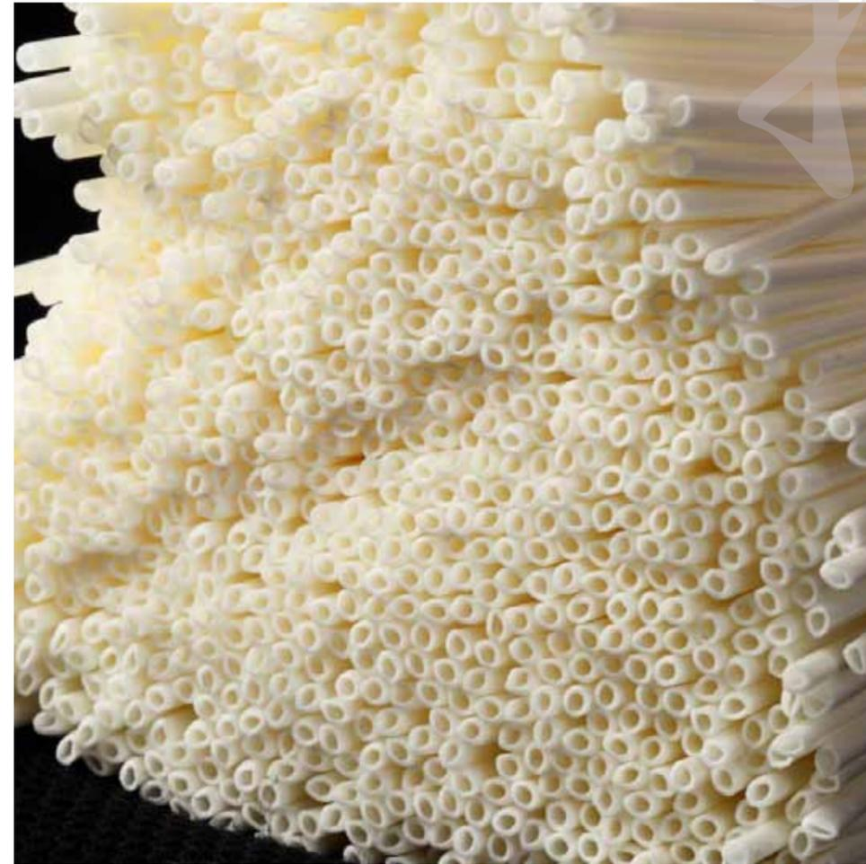
← Cross section of the membrane, the nucleus of the membrane-filtration system. Each membrane is like a straw. The 0.01-wide pores on the surface of the membrane fiber filter the water that passes through.
