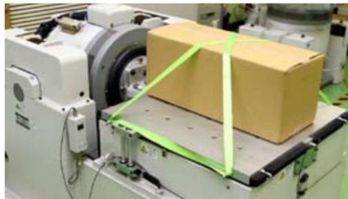
← The vibration test machine. Packaging can be tested at the level of vibration expected to occur during transport, to verify if there is any shifting or tilting of the contents, rupturing, or rubbing on the printed side. There are various other testing machines too.
