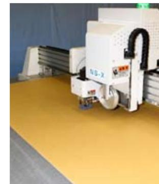
↑ Cardboard is trimmed on the sample cutter according to the design. The ability to make trial products in-house is one of the company's strengths.
