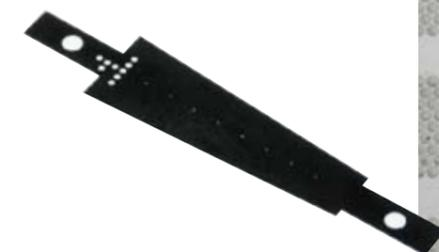
A sample of the micromachining that is Kumakura's base technology. (above) Orderly rows of 100 micron holes in the center of tungsten. (right) An example of the ultrasound technology that can be used to create requested patterns on materials of the customers choice, or perforate microscopic holes. The same kind of machining can be used on all kinds of optical glass, fine ceramics and quartz glass.
